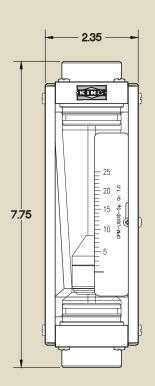
There is nothing else like it in the industry. This 75 mm scale glass tube meter offers economical 304 stainless steel case construction with vertical connections.
